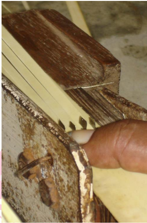
Photograph 7: Slicing the leaves using the m/c
