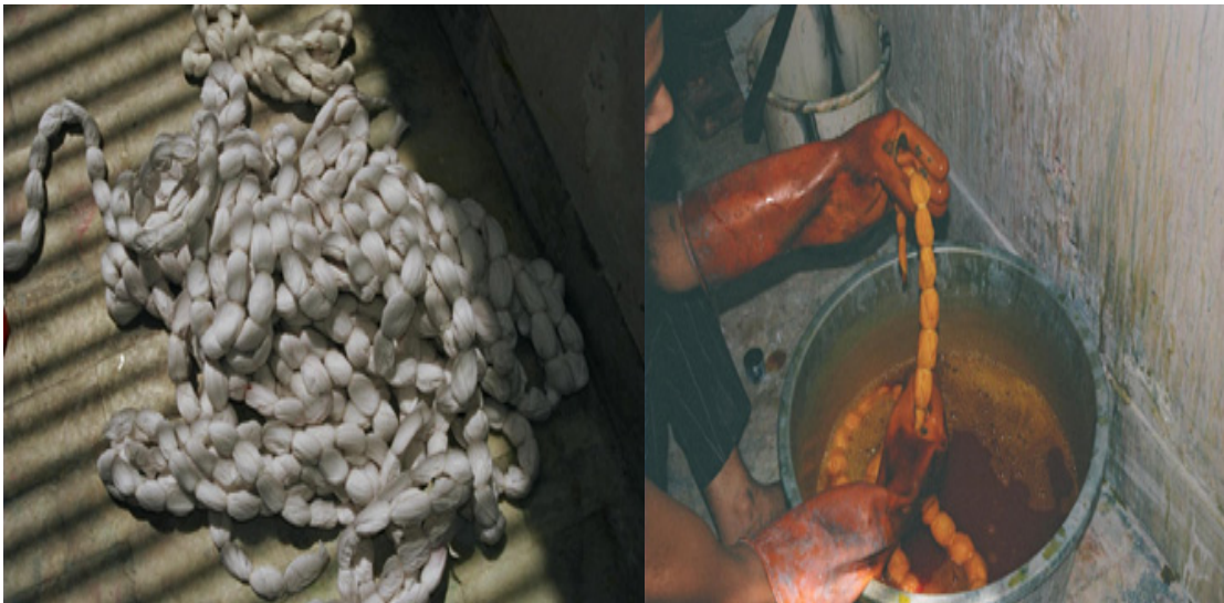
[Photograph 11 & 12: Showing leheriya tied diagonally being dipped]
