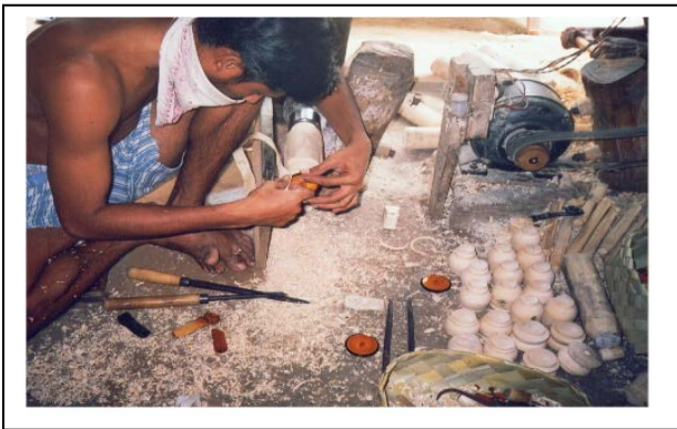
[Photograph: The artist is using emery paper for smoothing the semi-finished article]
