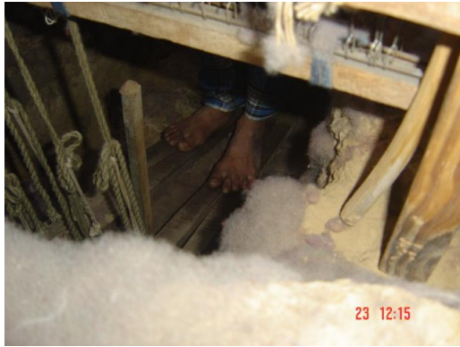
[Photograph 13: These pedals move the frames in an up and down movement]
