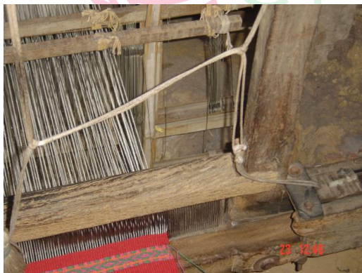
[Photograph 14: These pedals move the frames in an up and down movement]
