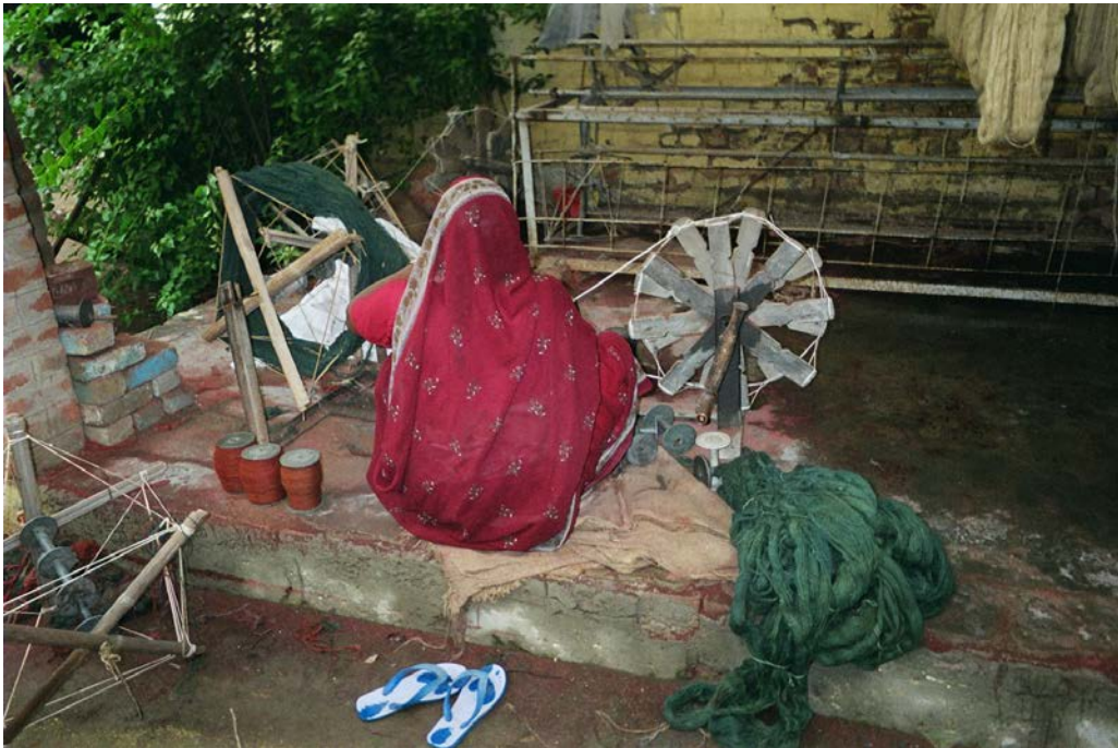
[Photograph 4: A charkha is used for making rolls or bundles of yarn for the weft].
