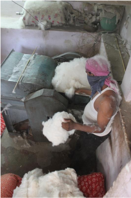
Artisan putting raw cotton on the cotton carding machine
