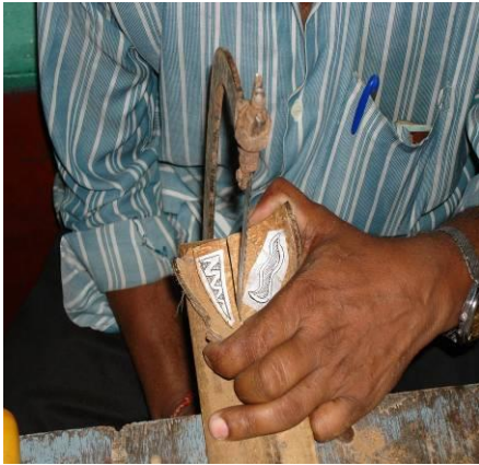
Photograph 13: Cutting out smaller pieces using hack-saw
