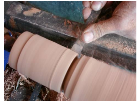
Photograph 21: Carving the design using a chisel
