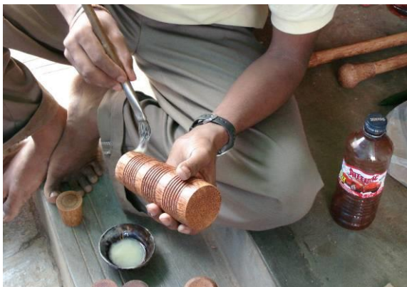
Photograph 25: Coating the piece with synthetic varnish
