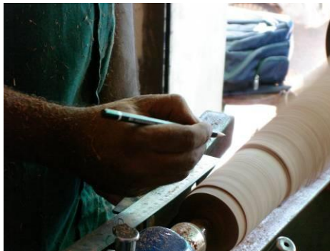
Photograph 20: Marking the design
