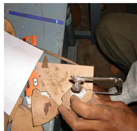
Photograph 12: Marking the design and cutting it out using bow cutter
