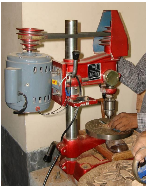
Photograph 7: Vertical drilling m/c
