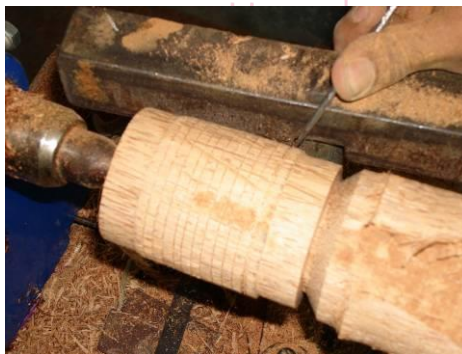
Photograph 23: Using fine chisel to give the detailing
