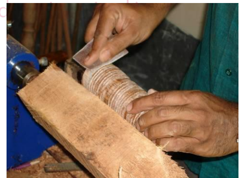
Photograph 24: Manually sanding the piece
