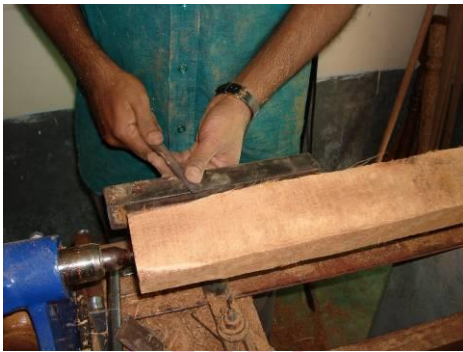
Photograph 19: Wood put on turning m/c and being cleaned, smoothened
