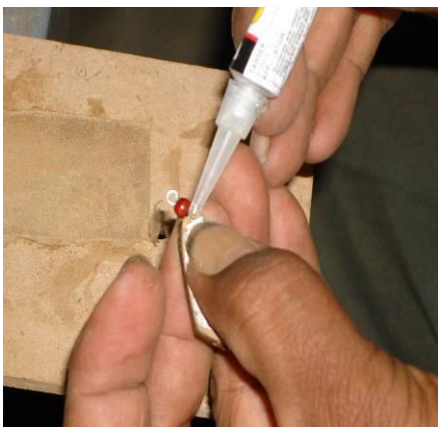
Photograph 16: Attaching hooks using adhesive
