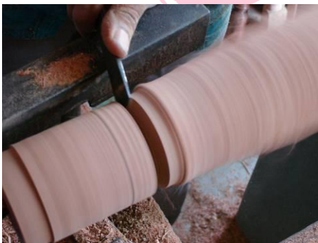
Photograph 22: Flat chisel being used to cut the piece
